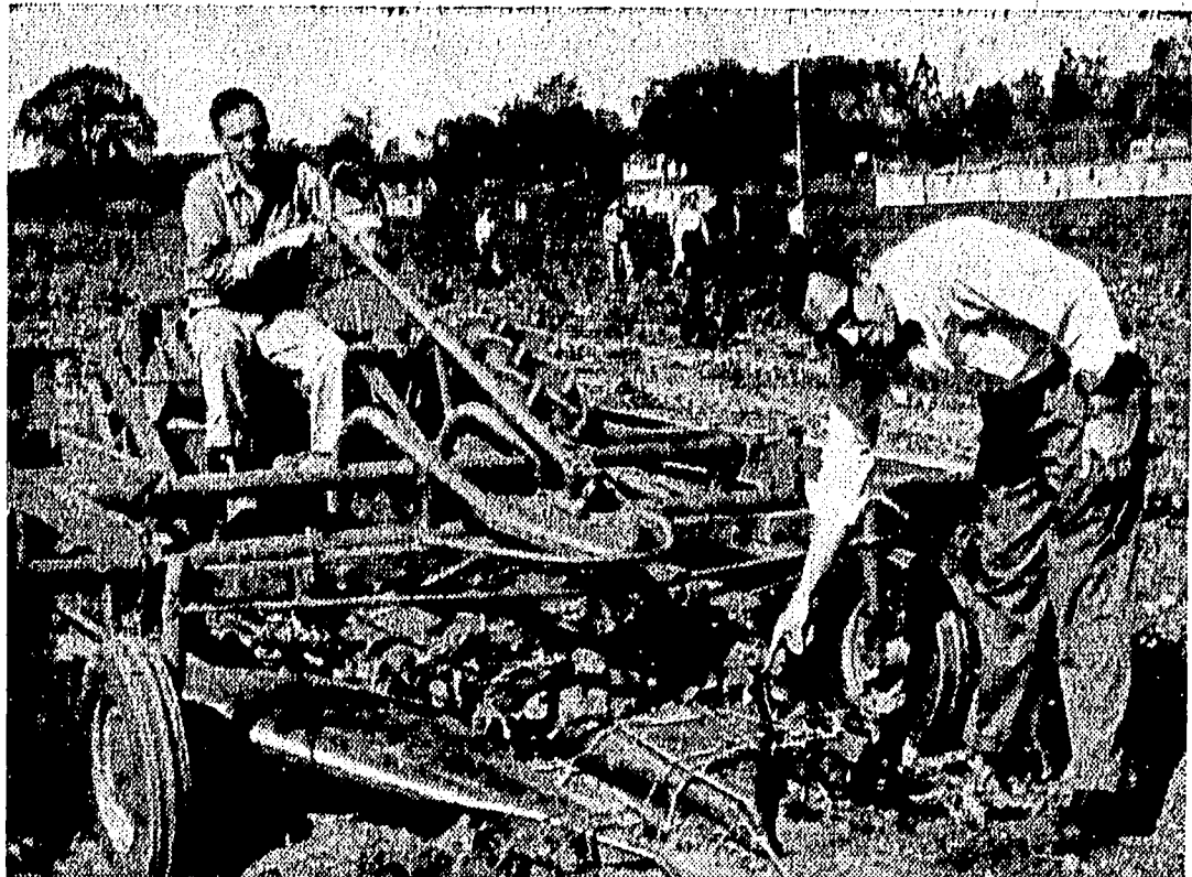
IF THIS MACHINE will work, a lot of Mexican braceros will be out of work. Dr. W. F. Buechle of the agricultural engineering department at Michigan State (standing) is demonstrating how the machine gently lifts the vines and picks all the cucumbers. George Bingley, student technician, is in the driver's seat. The machine operated experimentally gave promise. The picture was taken at the cucumber patch at the H. W. Madison Co. factory site in Mason. (Photo by M. H. Avery.)
