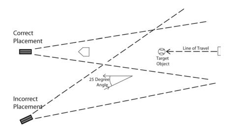
For accurate readings, the radar gun must be placed in the line of travel of the target. At slight angles, the error is very small; however, at larger angles, the error becomes substantial.
