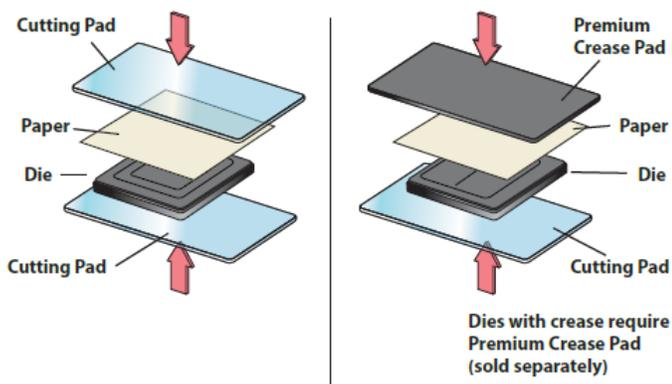
1. Place an Originals or Bigz die on a Cutting Pad with foam side up. Place paper or desired material to be cut on top of the die. Place the second Cutting Pad or Premium Crease Pad on top of the paper or material to create a "sandwich."
