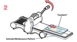
2. Place "sandwich" on Extended Multipurpose Platform and slide Platform into opening of Big Shot. Note the rotation of the handle and continue to rotate it in the same direction until the Platform has passed through the opening and the rollers. Remove Platform from Big Shot. Your die-cut shape is ready to use!
