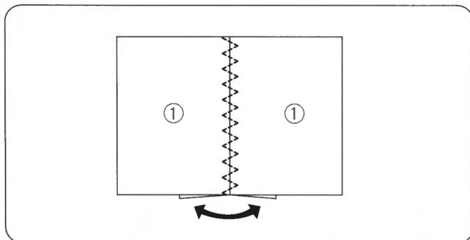
Place two layers of the fabric with the right side together. Seam along the edges with the straight stitch. Open fabrics flat and fold each seam allowances.
