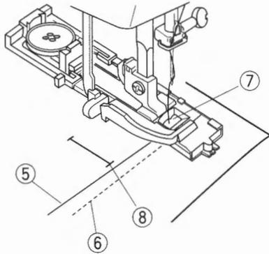
4 Raise the foot and pass the needle thread through the opening in the foot. Draw both needle and bobbin threads to the left.
