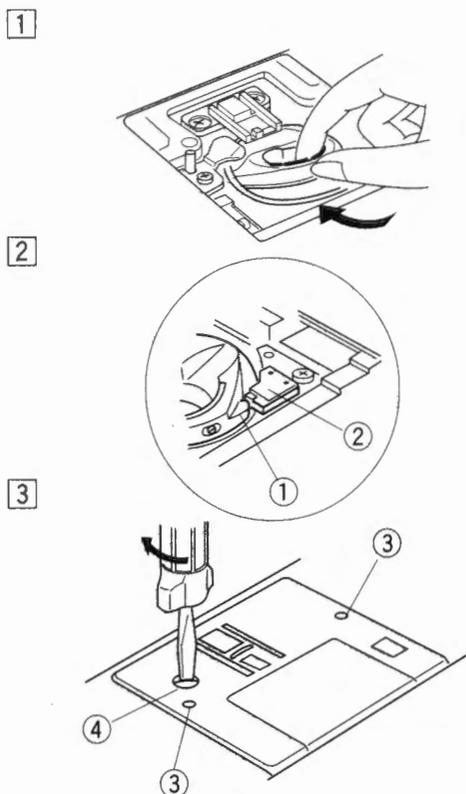
1 Insert the bobbin holder into the hook race.
