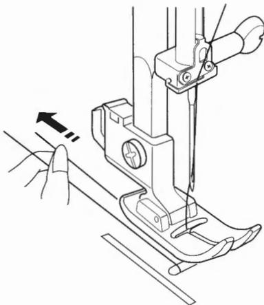
3 Pull 4" (10 cm) of both threads back and under the presser foot.
