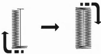
5 Sew slowly and stop the machine when a buttonhole is completed.
