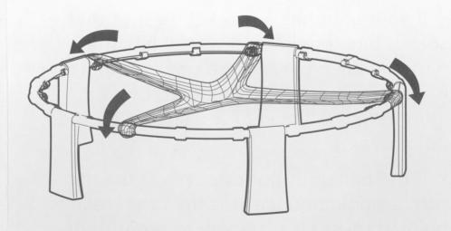
Spread out the net and attach it to the hooks in 4 places, making an "X" shape with the net. Note that the net goes over the rim and attaches to the hook underneath.
