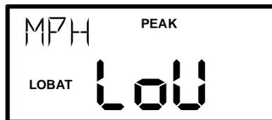
**NOTE:** WITH NiMH BATTERIES, DO NOT CHARGE THE BATTERIES UNTIL THE GUN DISPLAYS *LO BAT*.
