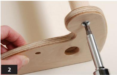
**15" Looms:** Align the center cross brace with the pairs of holes in the loom sides. Place a barrel nut into one of the holes in the brace with the slot on top and parallel to the long sides of the brace. Insert a 2" bolt through the loom side and screw into the barrel nut. Repeat for the remaining holes in the cross brace. **(Photo 2a)**
