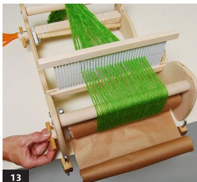
11. Continue rolling the warp and paper onto the warp beam. Stop every couple of full turns of the warp beam and pull firmly on the warp to tighten the warp and paper on the beam.
