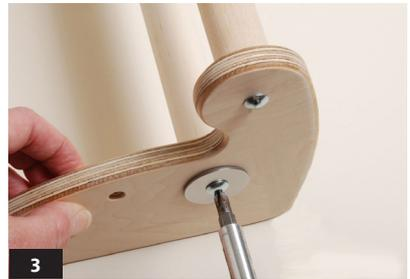
3. Insert and center the handles into the holes in the ends of the warp and cloth beams. If the dowels are a tight fit, use a hammer to gently tap them into place. Use the 3/8" screws to secure the handles. You can rub a bit of bar soap or paste wax on the screw threads to make them easier to turn, or use an electric screwdriver if you have one **(Photos 4–5 on next page)**.
