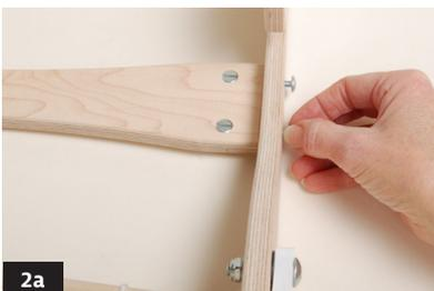
2. Working from the outside, insert the non-gear ends of the warp and cloth beams through the holes in the right side of the loom, then into the holes in the left side of the loom. Place a fender washer on each 1" screw and secure the warp and cloth beams on the left side of the loom. **(Photo 3)** Flip the ratchet dogs over so they sit on top of the gears.
