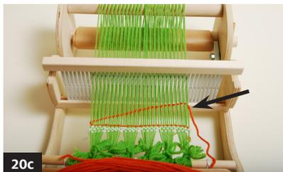
When inserting the weft into the shed, place it at about a 45 degree angle to prevent the weaving from pulling in at the edges (draw-in). (Photo 20c)
