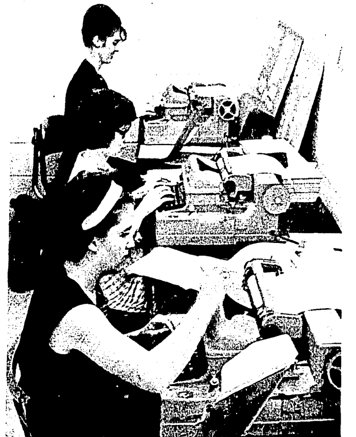
TURNING THE COPY into "type", offset style, is the responsibility of these 3 justwriter operators. Working on putting news onto perforated coded tape to be processed by other machines into reproduction proofs are, from front to rear, Judy Cole, Kathy Hausser and Sue Sanchez.
